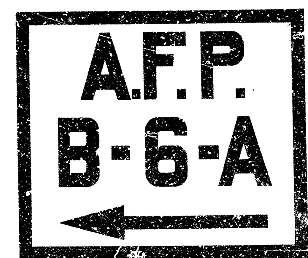
DETAIL OF MARKER PLATE TYPE AL-2 FOR FOREST HIGHWAY PROJECTS
